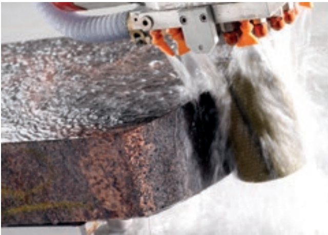
Grinding and polishing the edge of the slab.
