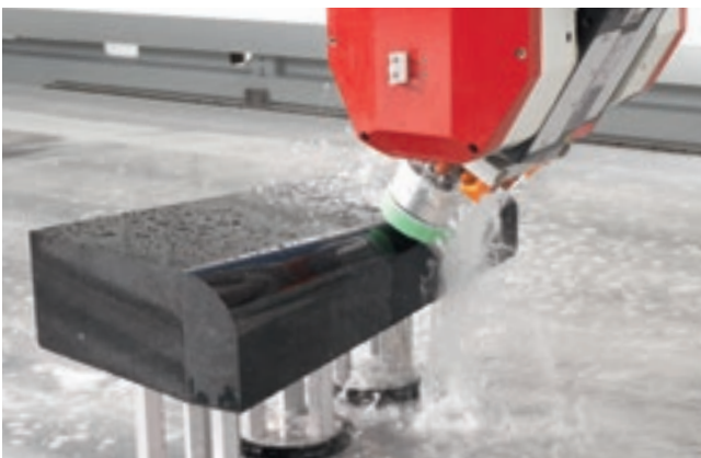
Polishing of rounded profiles on slabs.
