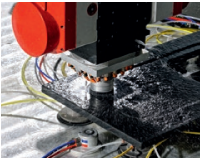
Flutes and recesses on kitchen tops, even with a tilted table.
