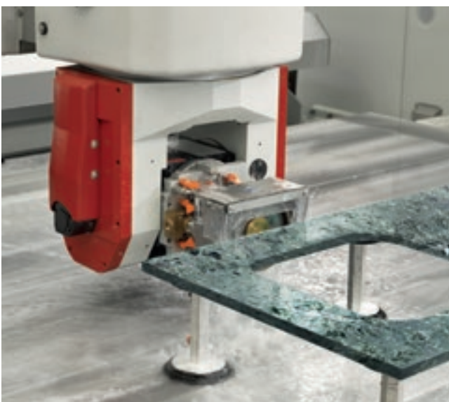
Cup grinding of the external edge.
